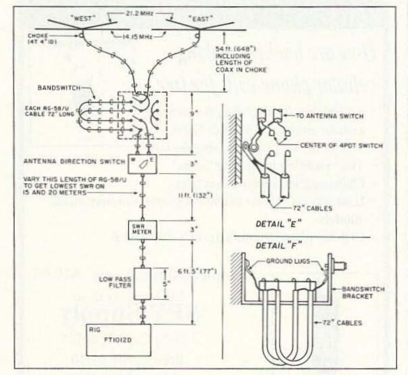
Figure. The corrected bandswitch diagram showing the proper switch connections.
